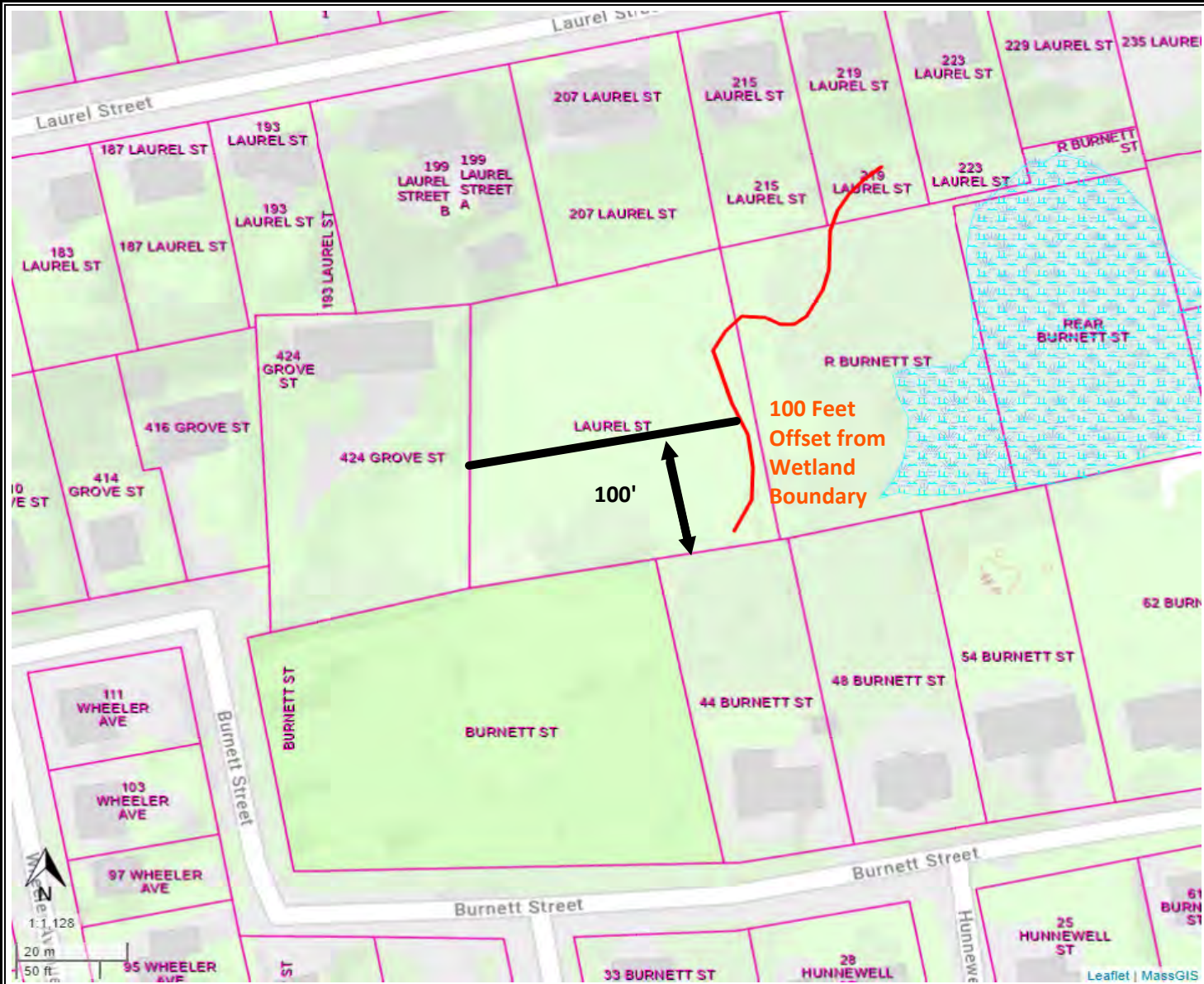
Notice of Intent Laurel Street Drainage Easement Pipe Replacement FIGURE 4 – Wetland Resource Boundaries (Assumed)
