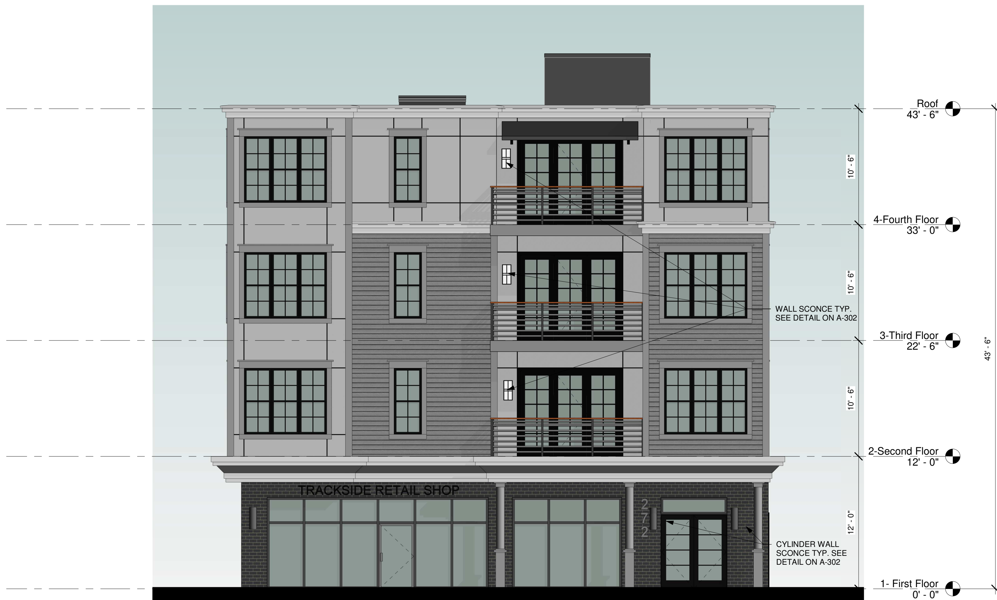
① Tremont Street Elevation 3/16" = 1'-0"
