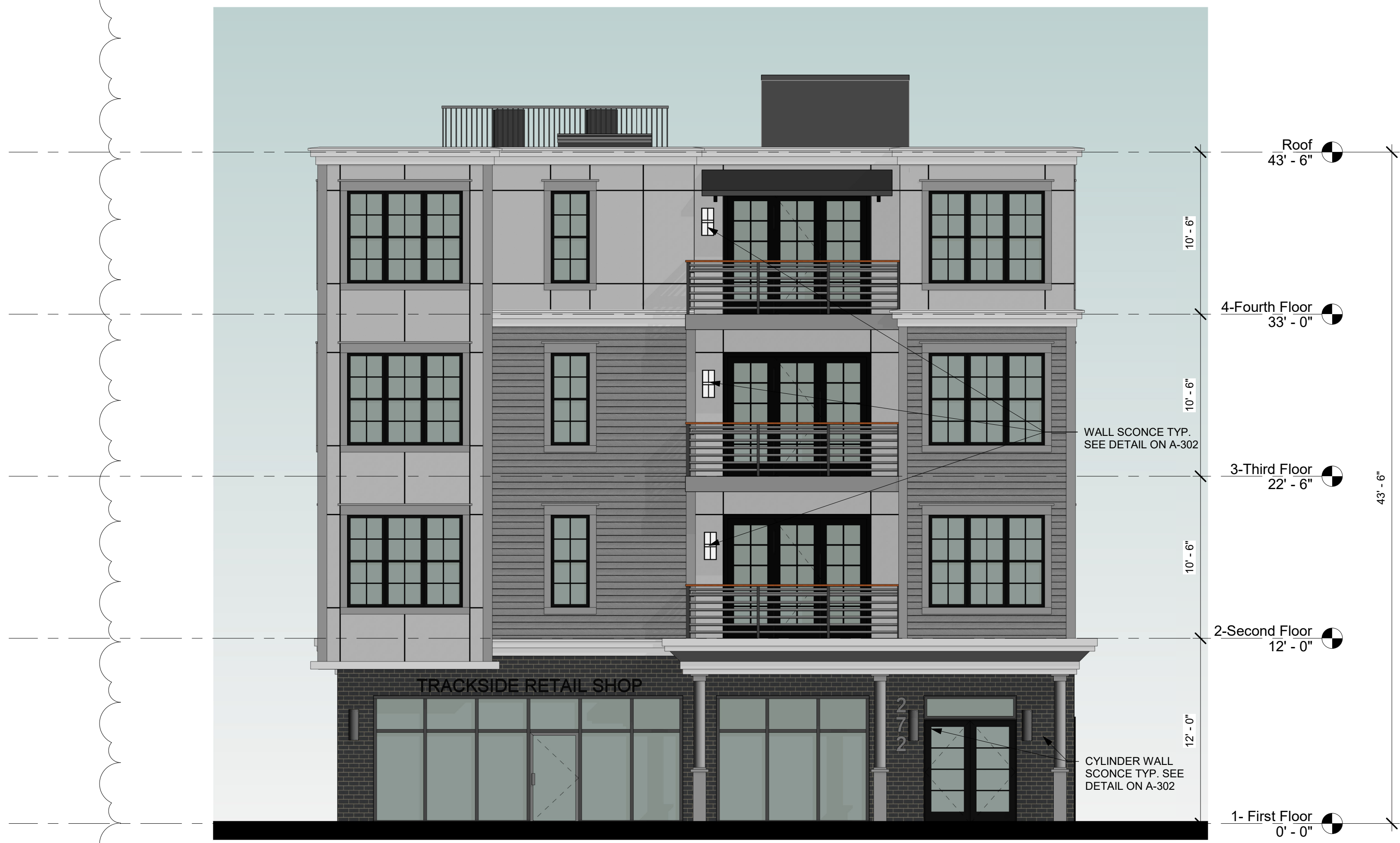
① Tremont Street Elevation 3/16" = 1'-0"
