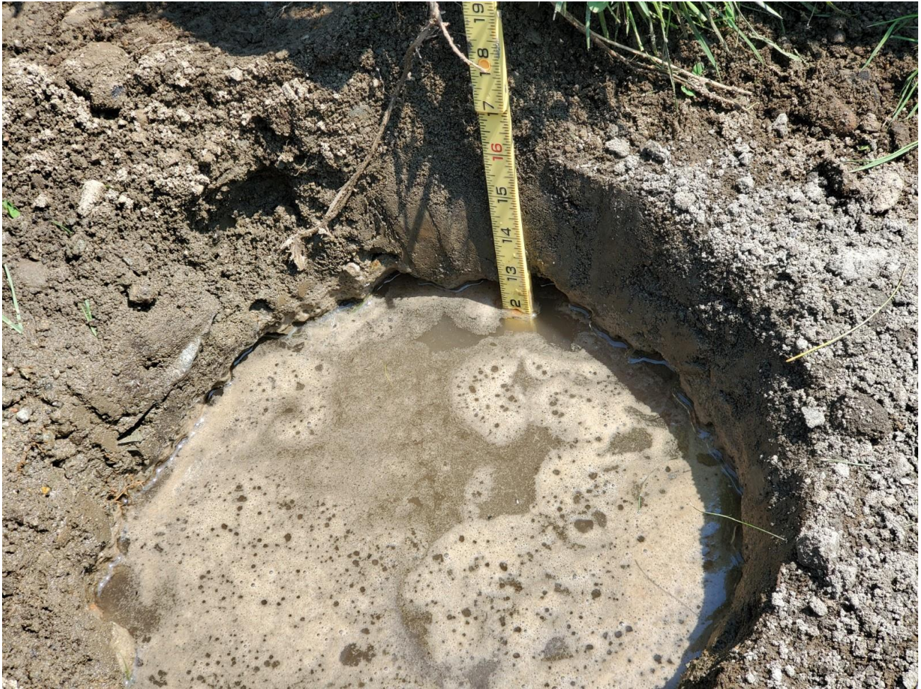
Photograph 4: Percolation Test in TP-8
