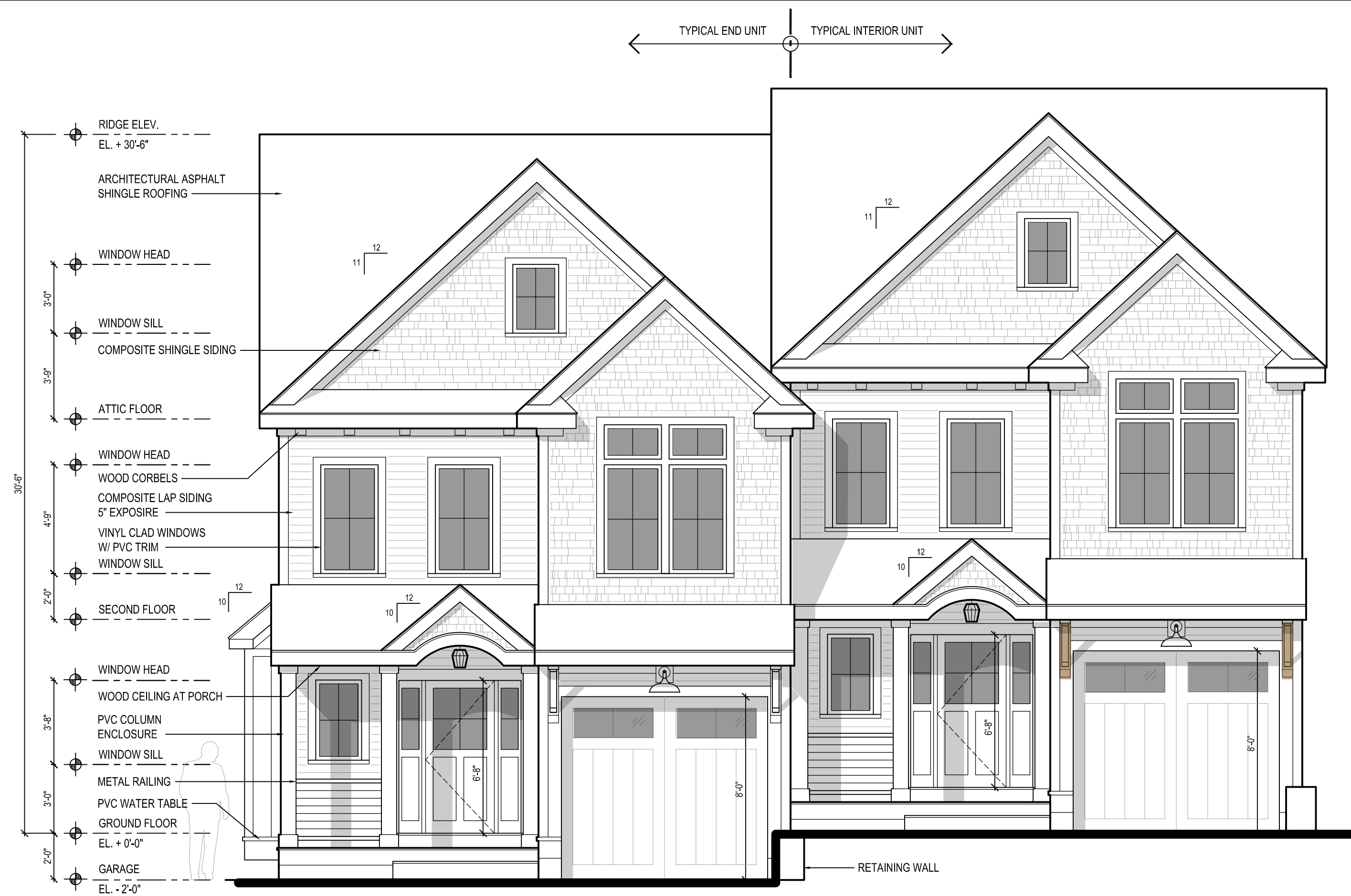
2 FRONT EXTERIOR ELEVATION SCALE: 1/4" = 1'-0"
