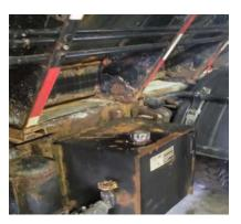
Conditions: Cracked frame. Rotted floor. Failed inspection.
