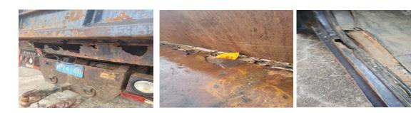
Conditions: Rotted floors and bed. Failed inspection.
