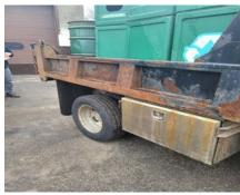
Conditions: Rotted floor and bed. Failed inspection. Primary vehicle to respond to pothole work orders.
