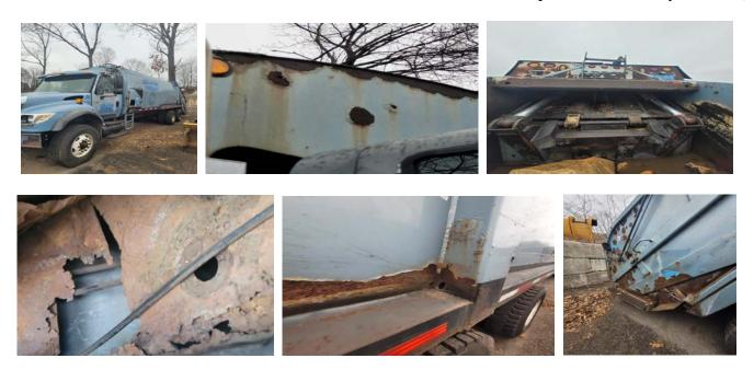
Conditions: Rotted body. Hydraulic lines in need of replacement. Rotted hopper.
