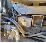
Conditions: Cracked frame in several locations has been welded and plated. Hydraulics in need of replacement. Passed most recent inspection but is not expected to pass in the future.
