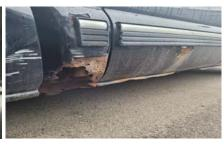
Conditions: Rotted Floor. Failed inspection.
