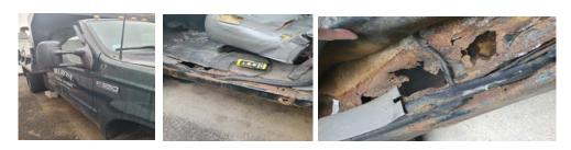
Conditions: Inoperable. Fire damage from recent vehicle fire during use. Rotted floor. Transmission
