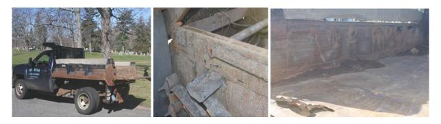
Conditions: Rotted body and bed. Failed inspection.
