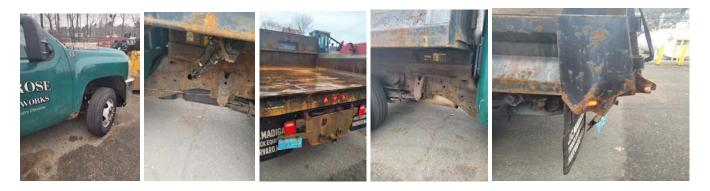
Conditions: Rotted floor. Failed inspection.
