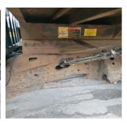
Conditions: Rotted holes in floor. Failed inspection. Primary vehicle for pulling landscape trailers and
