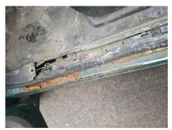
Conditions: Rotted Floor. Failed inspection.
